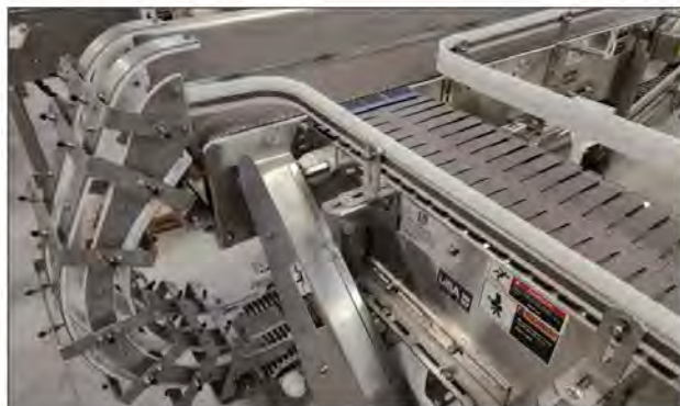
180-degree-gravity C-Chute-case-reorientation by Multi-Conveyor. © 2025 Multi-Conveyor
