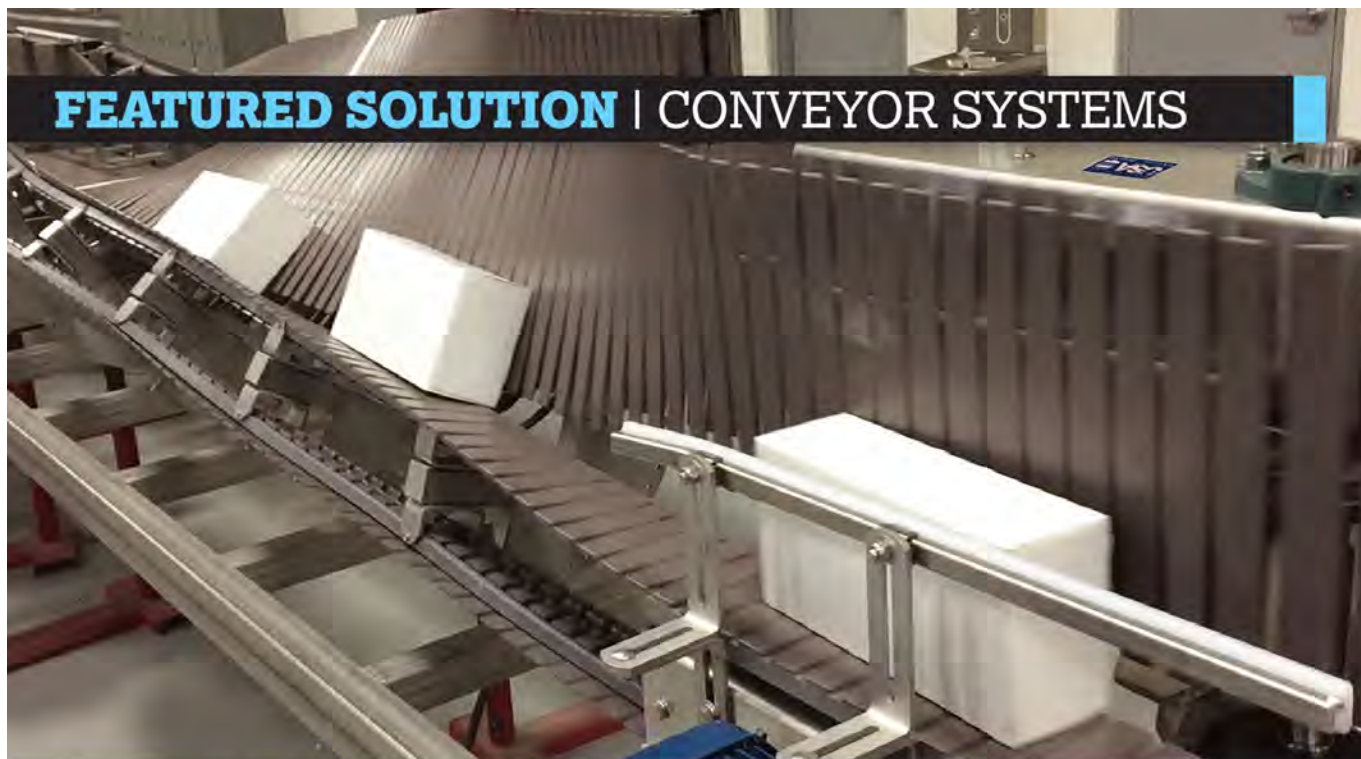
A Helix-Upender Twist-Conveyor for precision product rotation by Multi-Conveyor. © 2025 Multi-Conveyor
